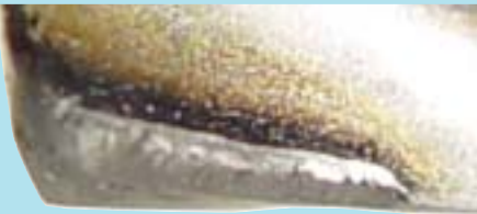
Carbide Tool Wear – Shrink Fit (bottom)
